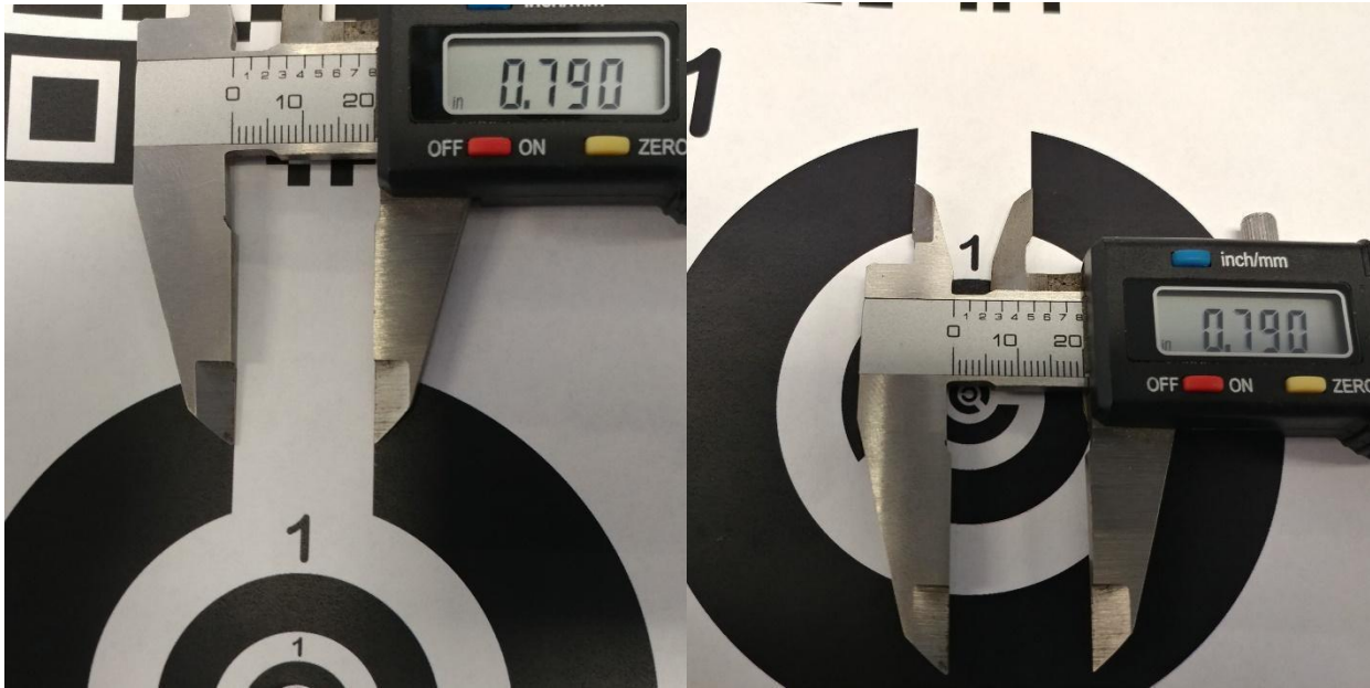
Figure 2 Outer Ring-Gap Measurement (1 of 5 on the sheet)
